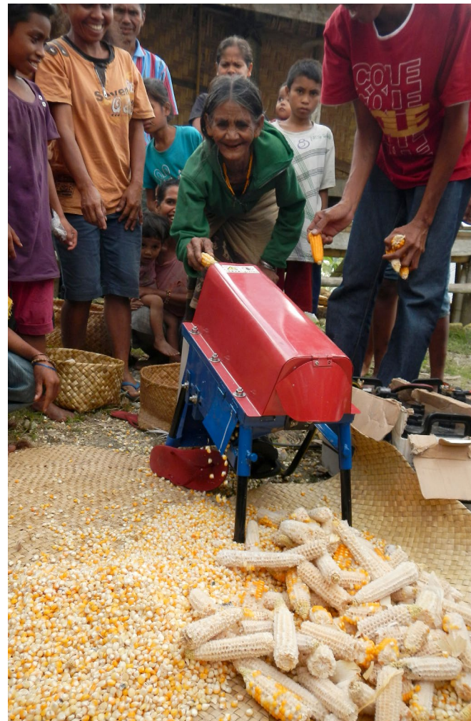
Solar PV-powered corn threshing in Vanuatu. Photo courtesy of Village Infrastructure Angels.
